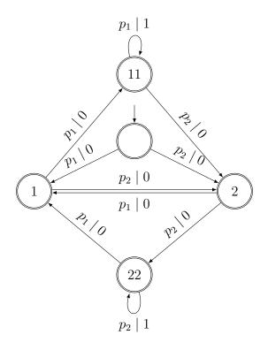
FIGURE 2. Transducer detecting the first 3-run of any letter.
